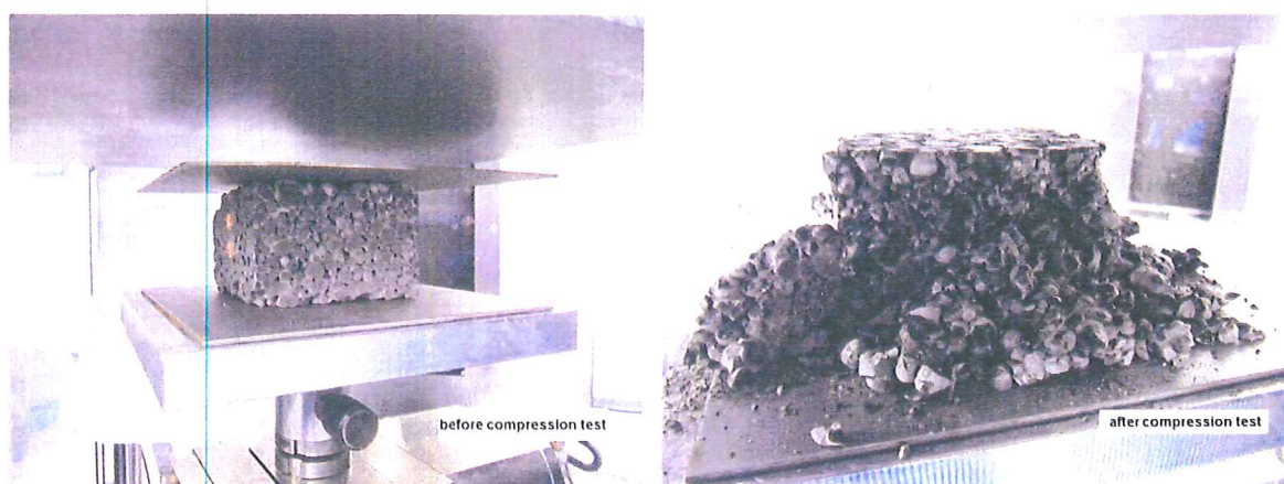
Figure 1: Test specimen; drainage mortar "LECADRAIN"
